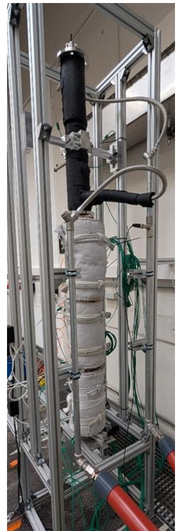
Fig. 1: Example of an experimental setup for high temperature heat pipe performance measurement.
