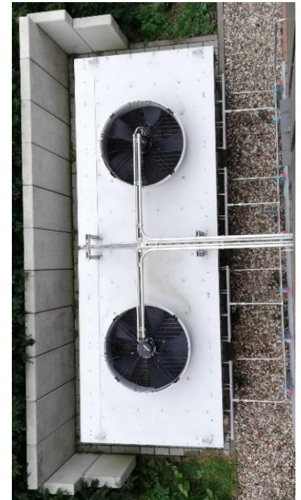
Figure 1: Air-cooled sCO 2 heat exchanger at the sCO 2 test loop in Essen, Germany
